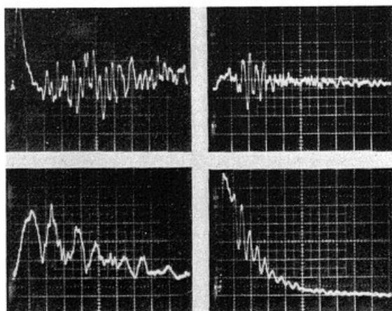
Fig. 3. Brain-implemented hydrophone responses to pulsed microwave irradiation in the cat (left) and guinea pig (right) at 5.655 GHz (top) and 2.450 GHz (bottom). Horizontal scale was 20  $\mu$ s/div. Vertical scales were 20  $\mu$ V/div for the cat; 100 and 200  $\mu$ V/div for the guinea pig at 2.450 and 5.655 GHz, respectively.
