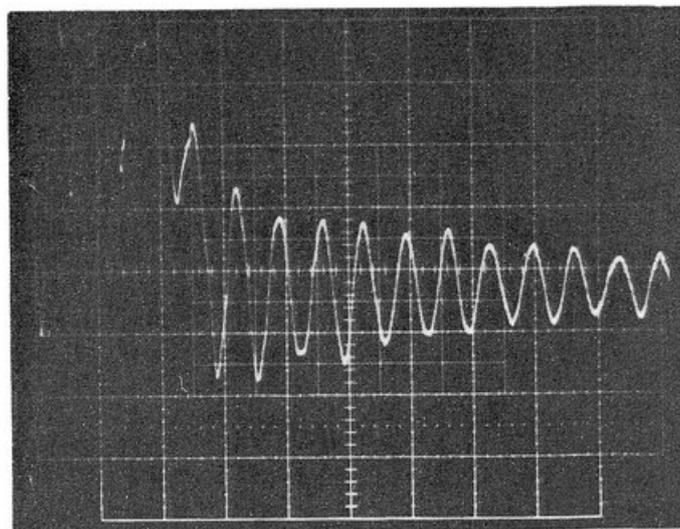
Fig. 2. Hydrophone response inside 6-cm diameter spherical brain model which was irradiated with a burst of three microwave pulses ( $10 \mu\text{s}$ ) at a 24-kHz rate. Vertical scale was  $100 \mu\text{V}/\text{div}$ ; horizontal scale was  $50 \mu\text{s}/\text{div}$ .
