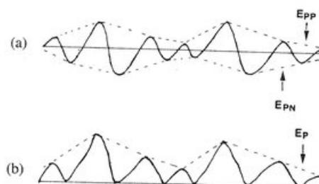
Fig. 5. (a) The envelope of positive peaks ( $E_{pp}$ ) and negative peaks ( $E_{pn}$ ). (b) The envelope of peaks ( $E_p$ ) after the baseline shifting ( $E_p = E_{pp} + E_{pn}$ ).
