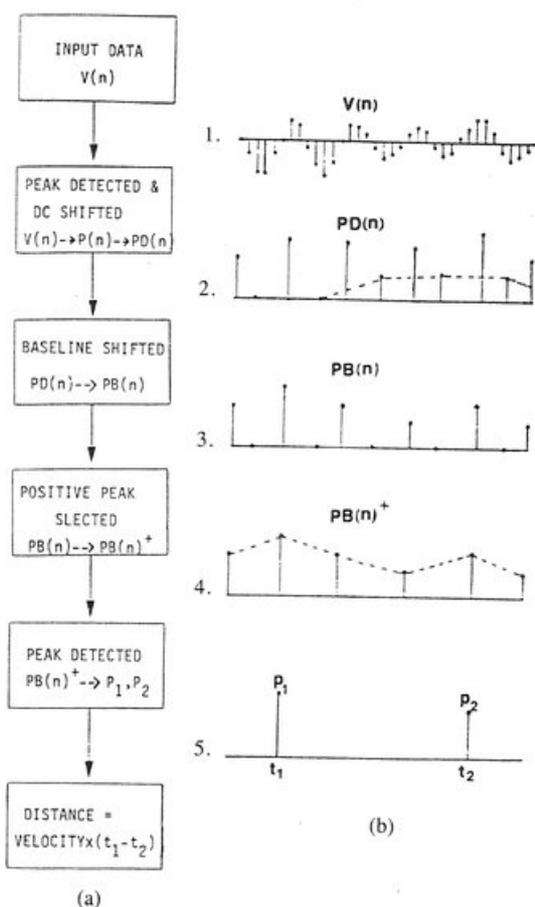
Fig. 3. (a) Flowchart for base-shifted, peak detection program. (b) An illustrative example.
