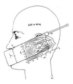
Figure 1 SAR measured inside a phantom human head irradiated by a flip cellular telephone with its antenna extended. The peak output power is 0.6 W. [From Balzano et al., 1995].
